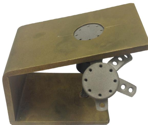
**Fig. 11.** To add internal screw threads to the holes on the upper surface of the pedestal anchorage base, a special clamp was designed, positioning the holes at a 17.5-degree angle.
